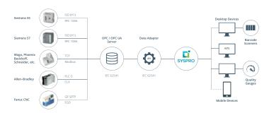
Depending on whether your machines are already data-enabled or not, you will either be able to extract the data directly from the machine, or you will need additional sensors that will need a sensor capable of capturing data in relation to the activities above. These sensors provide raw machine data which needs to be recorded centrally before being digitized and transformed into readable data.
